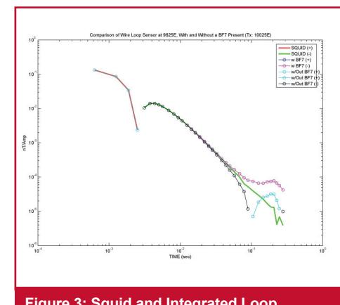
Figure 3: Squid and Integrated Loop Responses
