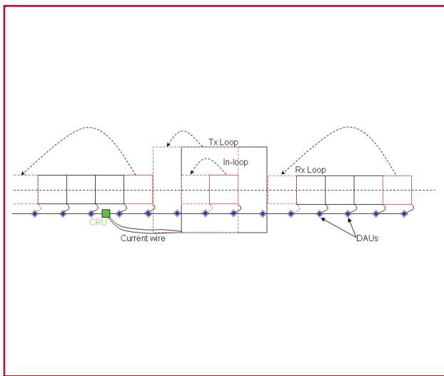
Figure 1: Example survey layout, using both in-loop and out-of-loop wire receivers.
