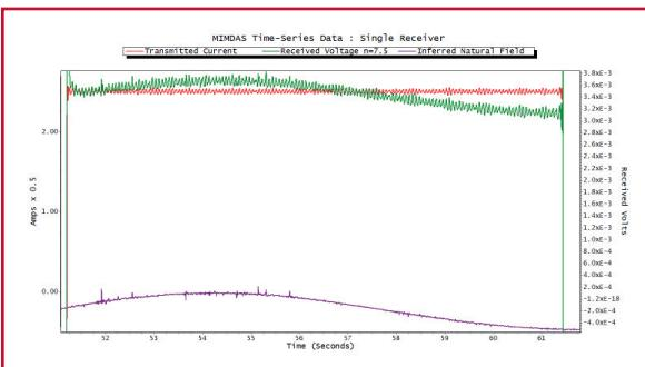
**Figure 4:** Blow-up of one on-period from the data presented in Figure 1. Cursory analysis indicates that the received signal (green) is corrupted by irregularities in the transmitted waveform (red) and a lively natural electric field (purple). The MIMDAS system is unique in its correct treatment of both corrupting sources.
